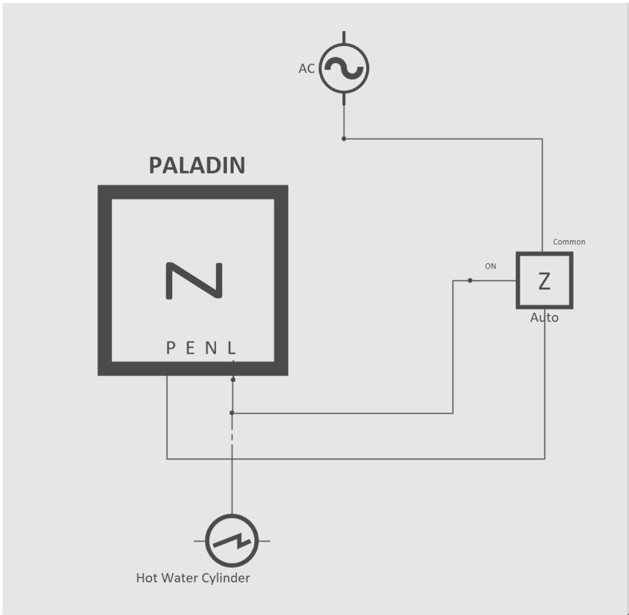
When Paladin is mounted next to the meter box, the temperature probe wire may need to be extended to the water cylinder. Use network Cat5 cable to extend the wire.
